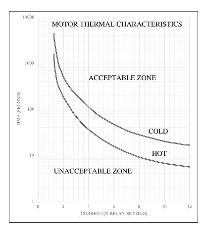
Motor Short-time Overload Withstand Characteristics (Is / In = 7.5)
