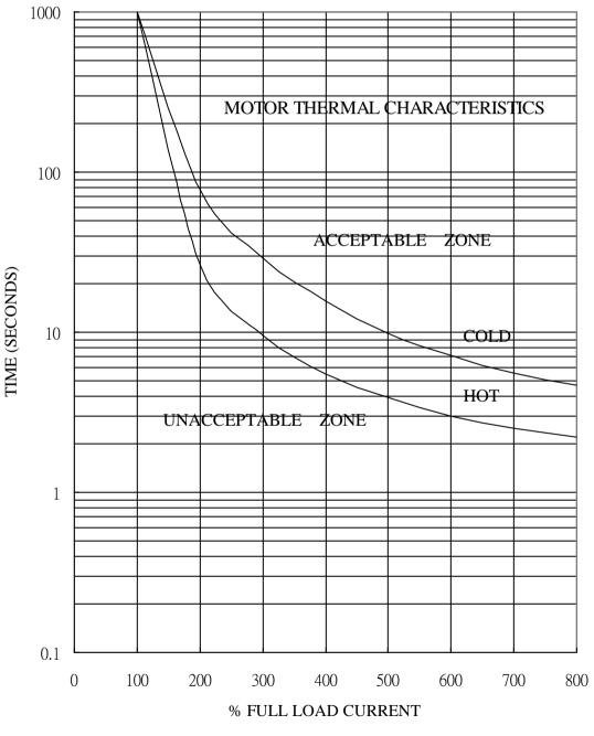
Motor Short-time Overload Withstand Characteristics
